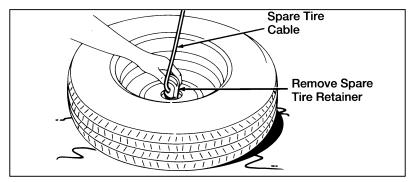
Removing the spare tire retainer
