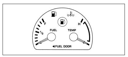
The engine coolant temperature and fuel gauge
