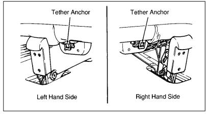
$\label{eq:figure 2} \textit{Figure 2: Tether anchor location} - \textit{second row bench seat (with built-in child safety seat)}$
