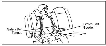
Figure 3: Shoulder safety belt placement on the child
