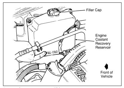
Engine coolant recovery reservoir fill location
