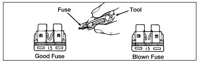
Fuse puller tool and fuse
