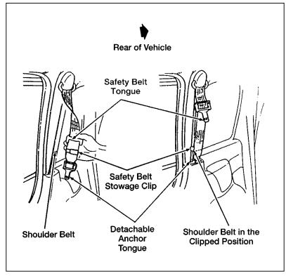
Figure 2: Securing the detachable shoulder belt
