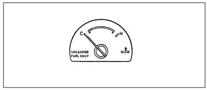
Engine coolant temperature gauge — base cluster
