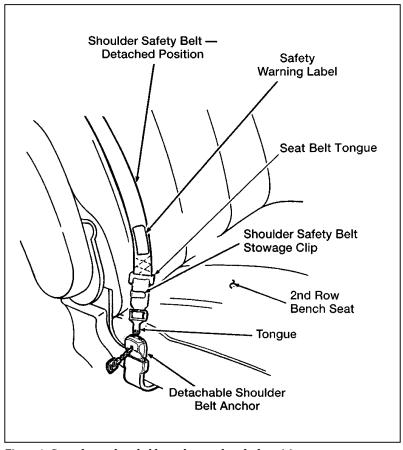
Figure 1: Second row detachable anchor — detached position
