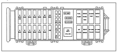
Engine compartment main fuse and relay panel
