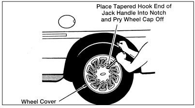
Wheel cover removal (optional cast aluminum wheels)
