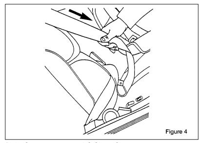
Setting the retractor to automatic locking mode
