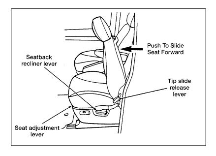
Push on the seatback to move the seat assembly forward. This provides access to the second row for loading and unloading groceries, briefcases, passengers, etc. through the driver's door.
