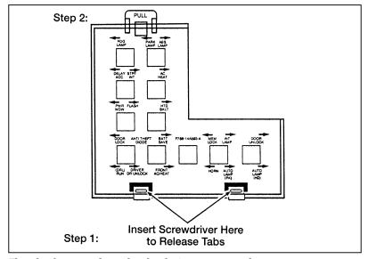
The relay box cover located under the instrument panel
