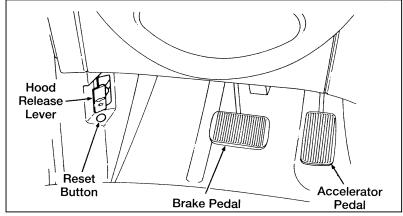
Fuel pump shut-off switch reset button location
