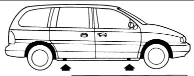
If your Windstar is equipped with accessory running boards, you must use the jack adapter when jacking the vehicle.
