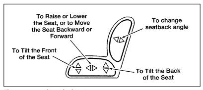
The power controls on the driver's seat
