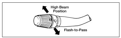
High beam and flash-to-pass operation
