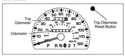
The speedometer, odometer and trip odometer
