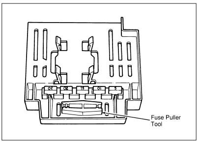
Fuse puller tool location — fuse panel cover
