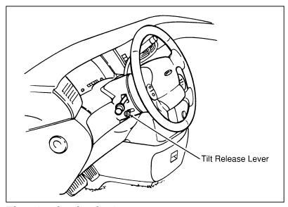
Tilt steering release lever location
