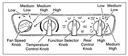
The climate controls — main and auxiliary system A/C — Heater System — if equipped
