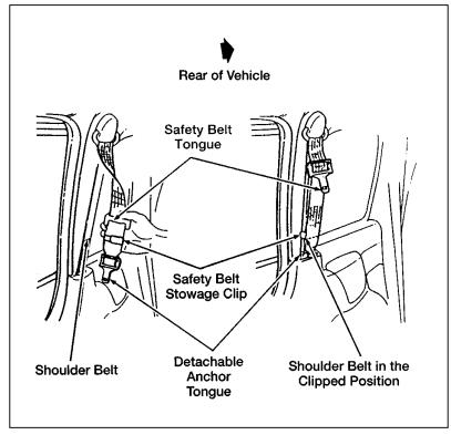
Figure 2: Securing the detachable shoulder belt
