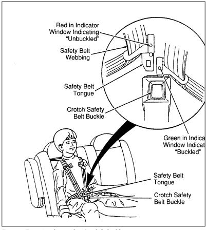
Figure 4: Fastening the crotch safety belt buckle
