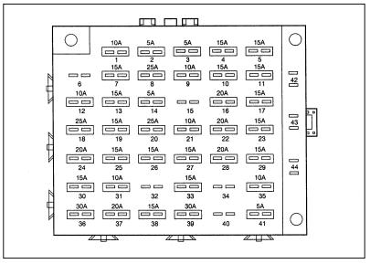
Main fuse panel under instrument panel
