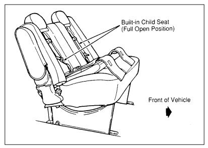
Figure 1: Built-in child seat fully open
